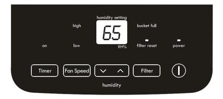
6. The TIMER function enables you to either Delay Start or Delay Stop the unit in the choice from 0.5 hour to 24 hours. If the unit is running, then selecting Timer will turn the unit off after setting hours (Delay Stop). If the unit is off, then selecting Timer will turn the unit on after setting hours (Delay Start).
